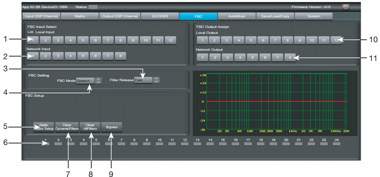
The Feedback Canceller function automatically eliminates the feedback produced by microphones to nearby loudspeakers.
