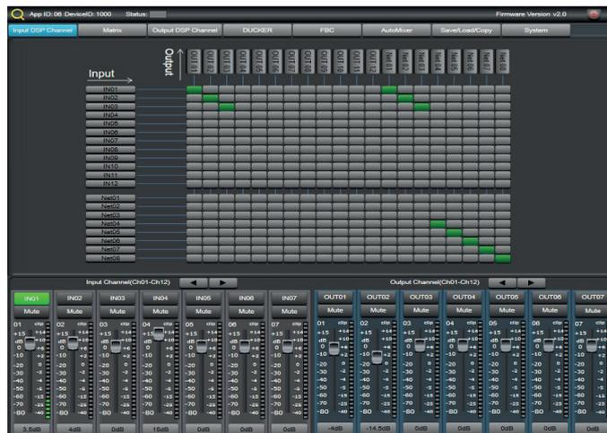
In this image, analogue input channels 1, 2 and 3 have been assigned to analogue outputs 1, 2 and 3 of the matrix and input channels 1, 2 and 3 have been sent to NET channels 1, 2 and 3.
