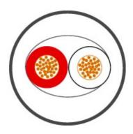
OFC cable with double insulation
